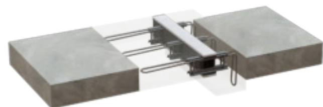
Anchoring downwards into a reinforced concrete beam; minimum dimensions of the beam: width – 180 mm, height – 360 mm.
