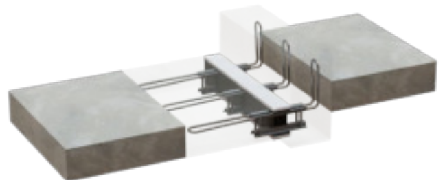
Anchoring upwards into a reinforced concrete beam; minimum dimensions of the beam: width – 180 mm, height – 360 mm.
